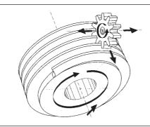
The process is divided into a roughing and a finishing operation. A specific software package provides a variety of standard options for selection (e.g. multiple-flank roughing, dual-flank finishing) and cycles (e.g. random indexing cycle). The precise positioning of the grinding wheel is supported by a special function in the software and this considerably reduces set-up time.
