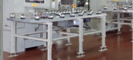
Machine with NC gantry loader, lifting capacity per gripper of 7 kg. Continuous indexing chain belt with central lifting station for supplying blanks and discharging finished parts.
