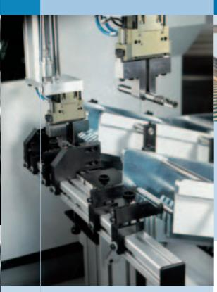
The combination of indexing chain belt and V-magazine for supplying blanks and the unloading belt for discharging finished parts provides another interesting option for rapidly changing over long shafts, pinions and gears.
