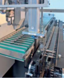
Cylindrical shafts placed in and removed from stacks by lifting loader. This automated solution provides a high level of autonomy for little space. Fast and flexible workpiece loading/ unloading systems are available for the P 90 G.
